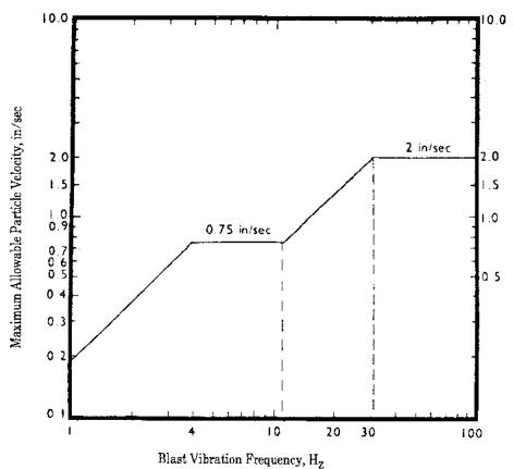
Figure 1. Alternative blasting level criteria.
