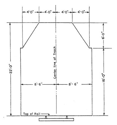
$Figure \ 2. \quad General \ Clearance \ Diagram \ for \ Buildings \ Adjacent \ to \ Tangent \ Track \ on \ Steam \ and \ Diesel \ Railroads.$
