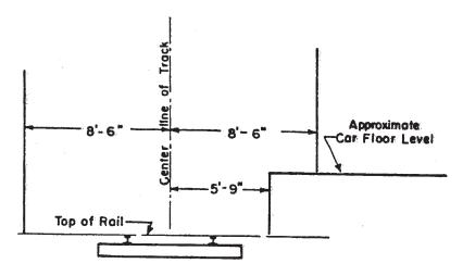
Figure 4. Clearance Diagram for Freight Platforms, Retainers and Guards Adjacent to Tangent Track on Steam and Diesel Railroads
