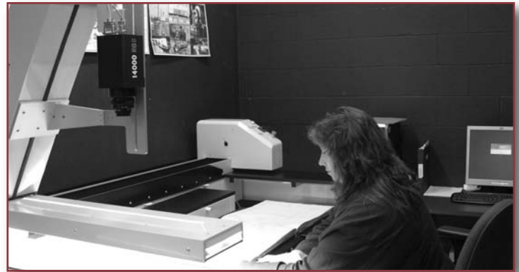
Stacy White uses a planetary scanner to image oversized and bound materials.
