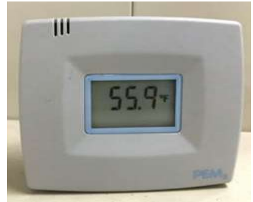
An example of a data-logger which can measure both temperature and humidity.
