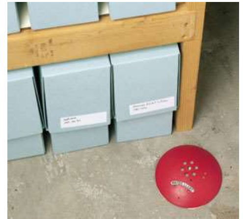
An example of a floor water sensor that will alarm during flooding
